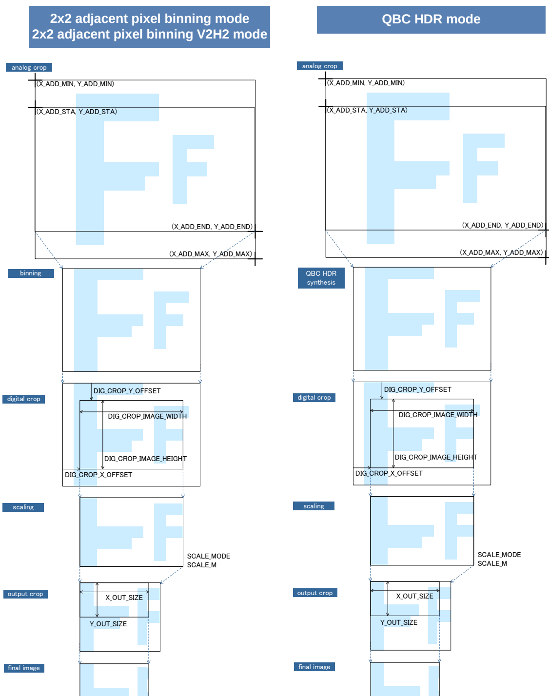
Figure 15 image area control capabilities for 2x2 adjacent pixel binning mode, 2x2 adjacent pixel binning V2H2 mode and QBC HDR mode
